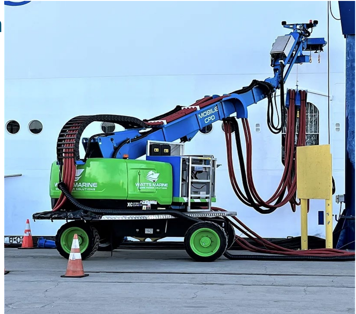
Mobile Cable Positioning Device (CPD)
